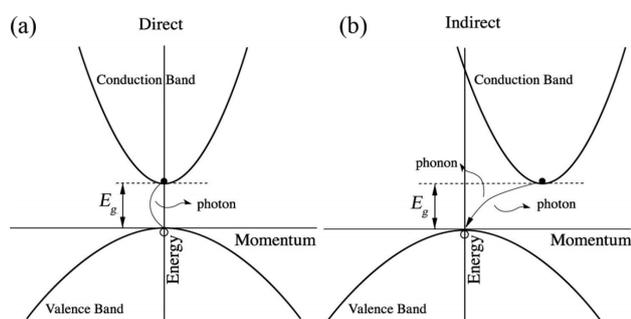
**Figure 2.** One-dimensional band diagrams containing (a) direct and (b) indirect bandgaps
