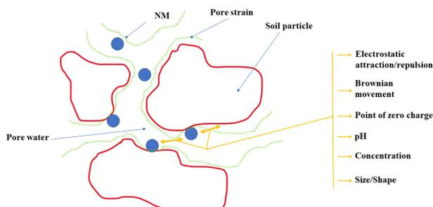
**Figure 6.** Schematic diagram representing the factors which effect the dissolution/transport of nanomaterials between soil and pore water
