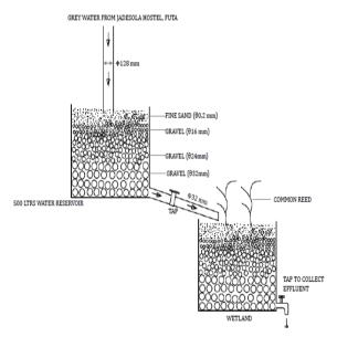
Figure 1. Greywater Treatment Setup
