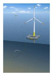
Figure 6. Floatgen and its mooring system<sup>[18]</sup>
