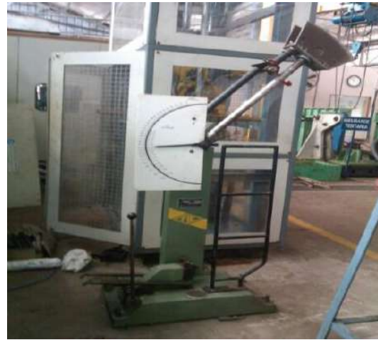
Figure 1. (e) Charpy impact tester
