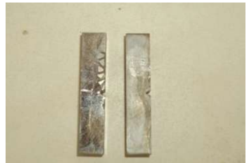
Figure 1. (f) 20 \mu Samples of Ni and Cr corroded for 2400 hours.
